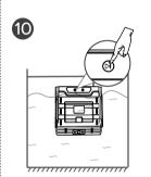
• Press the (>) button to start the pool cleaning.
