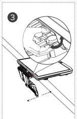
Adjust the angle screw height to ensure the hook press against the wall tightly, and tighten it after fixing.
