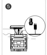
Connect the cable from the solar kit to the one from the docking station. and insert the connector into the groove.
