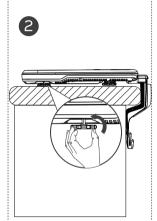
Adjust the height of the level screws on the bottom of the solar kit. ensuring the solar panel on the deck is flat enough.
